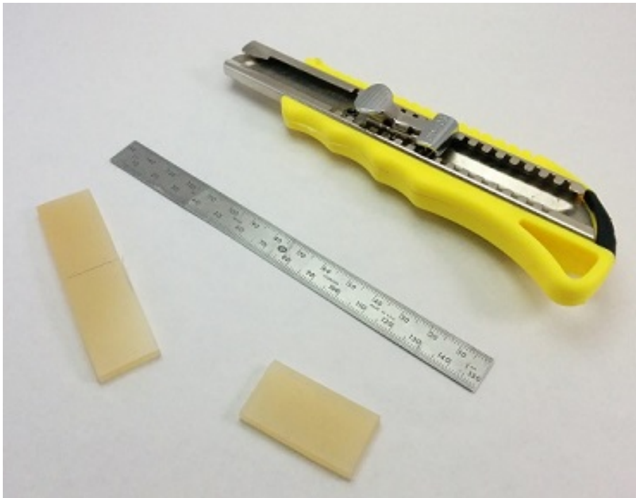
Cutting the silicone sheets with a cutter and a ruler.
