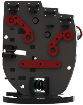
Fig. 3. Inner side of the palm. The three bars of the proposed whiffletree are depicted with red color. The holes of the upper two bars are filled by the elongated parts of the corresponding buttons, constraining the motion of different fingers. In this instance the motion of the index and pinky fingers is constrained, resulting to a change at the inclination of the differential mechanism finger bars.
