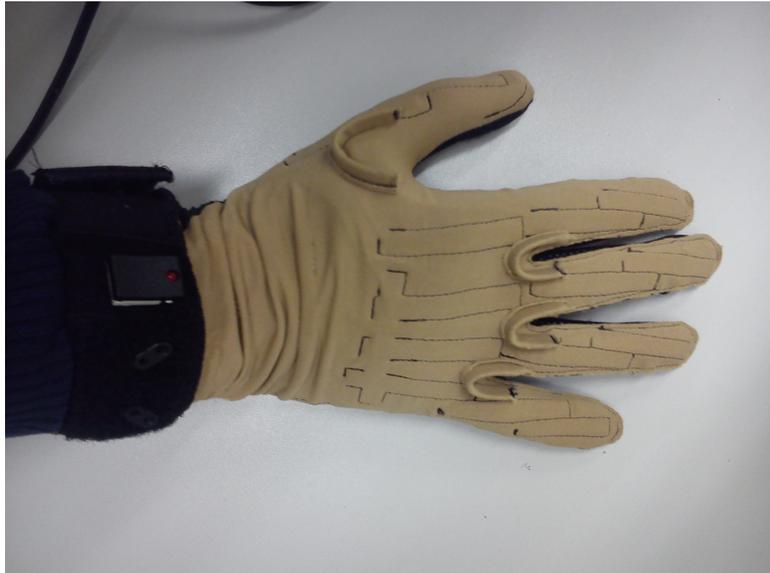
**Figure 5.1** – CyberGlove II, CyberGlove Systems [6].
