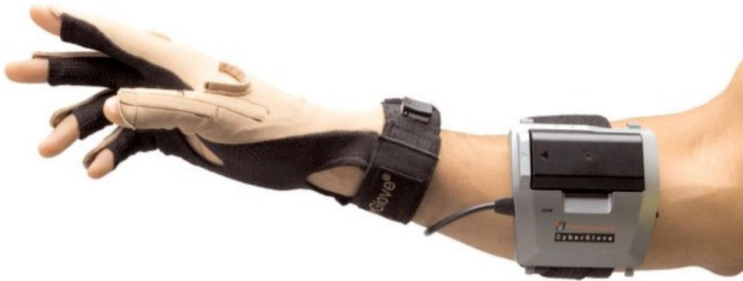
**Figure B.1** – CyberGlove, a glove which captures human hand’s kinematics in real-time mode [6].
