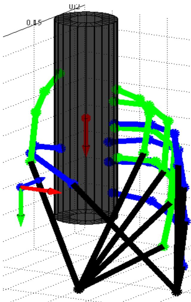
**Figure 4.7** – Joint angular displacements as decision variables: Initial (blue hand) and final (green hand) posture of the robot hand.
