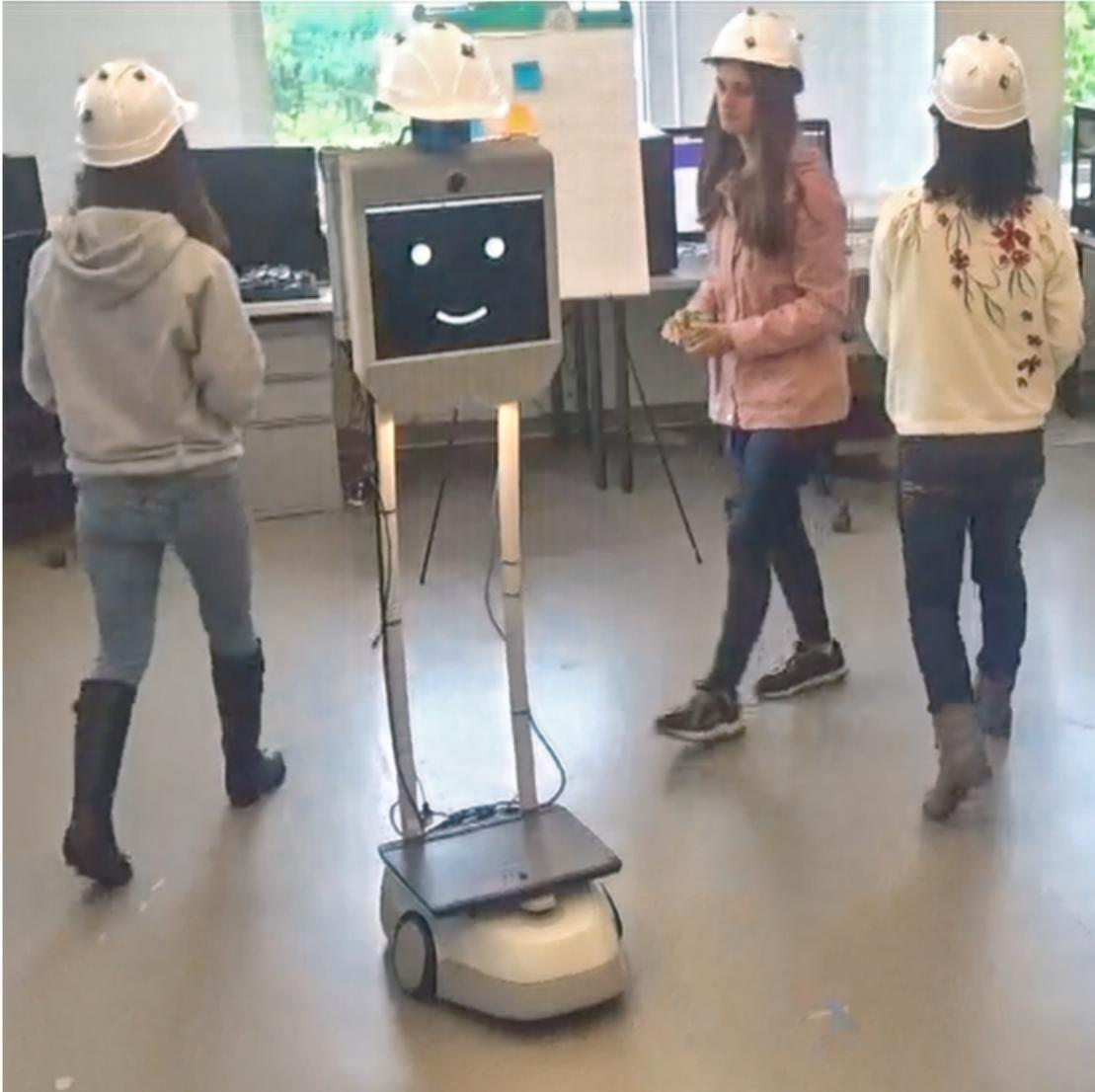
**Figure 6.1: This study examines the performance of autonomous robot navigation algorithms in crowded pedestrian spaces.**
