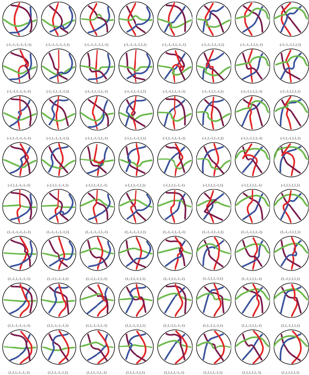
**Fig. 7.** Top view of trajectories generated by executing the same four-agent scenario with all possible topological specifications. The subcaptions denote the topology tuple that was used as a specification for each execution.
