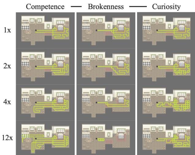
**Figure 5: Robot trajectories that communicate desired attributions generated by our trajectory optimization framework [34]. Columns indicate the type of attribution and rows indicate the intensity of the attribution.**
