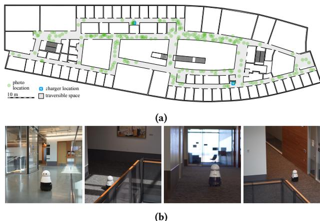
**Figure 2: Our Kuri robot wandered a  $28,000ft^2$  floor for 4 days with minimal human help [23]. (a) Kuri’s coverage of the building floor. (b) Photos of Kuri as it wandered in the environment.**
