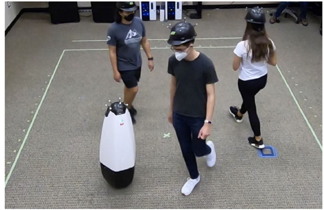
FIGURE 1 Honda's experimental ballbot (Honda 2019) navigates next to three users in our lab experiment (Mavrogiannis, Balasubramanian et al. 2023).
