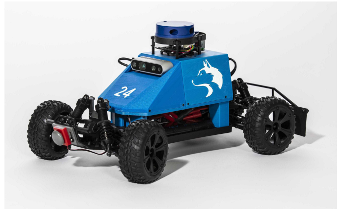
Fig. 1: The MuSHR racecar. MuSHR can be built for $600, through the use of off-the-shelf components, and user-friendly build instructions, found at our website, ( https://mushr.io ). A complete open-source software stack can be found at our Github pages, ( https://github.com/prl-mushr ).
