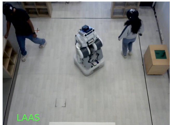
Figure 1: Still from our experiments. Two users and a robot are navigating in a constrained workspace. We mirrored the same study setup at UM and LAAS, using a Hello Robot Stretch (left), and a Willow Garage PR2 (right), collecting interactions with a total of N = 80 subjects. A video supplement with excerpts from our experiments can be found at https://youtu.be/QGd5vQMhXqY .
