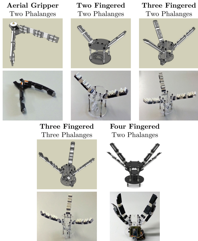
Figure 9: Different robot hand models and robot hands created with the design directions provided, are depicted.
